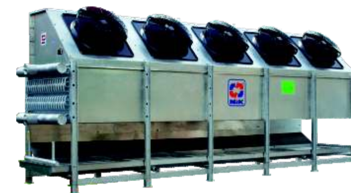
Spiral Freezer Ammonia Unit Cooler AND-S Capacity Range 28.6 to 365.9 kW Fan Diameters 630 or 710 mm No of fans 2, 3, 4 or 5 Fans Fin Spacing 6, 8, 10, 12, 15 or 12/15
