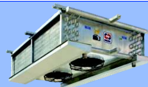
Dual Discharge Ammonia Unit Cooler AND-D Capacity Range 3.5 to 65 kW Fan Diameters 400, 450, 500, or 560 mm No of fans 1, 2 or 3 Fans Fin Spacing 6, 8, 10, 12, 15 or 12/15
