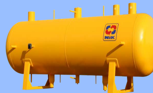
Ammonia Intermediate Cooler NLSI Diameter Range up to 2 m Length Range up to 12 m Temperature Range -50 to 50°C Working Pressure Range up to 20 bar
