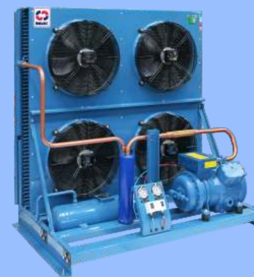
Refrigeration Condensing Unit NUC Heat Rejection Capacity 4.4 to 175 kW Suitable Compressors 1 to 27 hp Fan Diameter 350, 400, 450 or 500 mm No of Fans 1 up to 6 Fans
