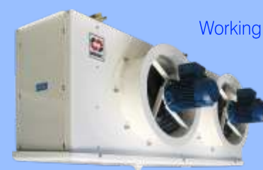
Explosion proof Unit Coolers Capacity Range 1.7 to 76.7 kW Fin Spacing 4, 6 or 8 mm No of Fans 1, 2, 3 or 4 Fans Fan Diam. 350, 400, 450 or 500 mm
