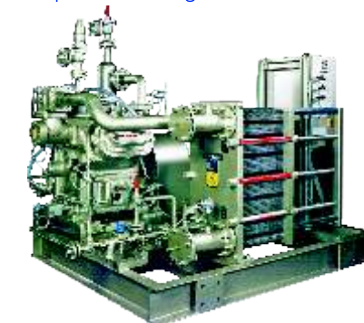
MAYEKAWA Reciprocating Chillers Capacity Range 41 to 677 kW Refrigerant: Ammonia or Freon Temperature Range +12 to -30°C
