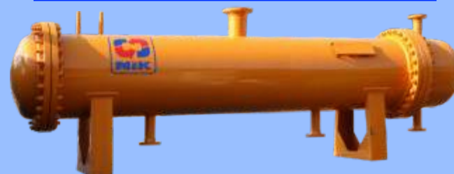
Shell & Tube Heat Exchangers NSTE Diameter Range up to 2m Length Range up to 6m Temperature Range -50 to 150°C Capacity According to the order
